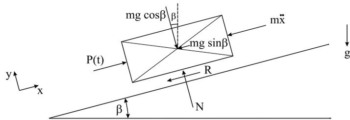
$$\begin{pmatrix} P(t) - mg \sin \beta - R \\ -mg \cos \beta \end{pmatrix} + \begin{pmatrix} 0 \\ N \end{pmatrix} + \begin{pmatrix} -m\ddot{x} \\ 0 \end{pmatrix} = 0 \quad (1)$$
