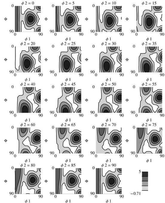
Fig. 3. Approximation of the codf based on  $V'_{(4)}$ ,  $V'_{(6)}$ , and  $V'_{(8)}$ :  $\bar{f}(\mathcal{Q}) \approx 1 + V'_{(4)} \cdot F'_{(4)}(\mathcal{Q}) + \dots + V'_{(8)} \cdot F'_{(8)}(\mathcal{Q})$ .
