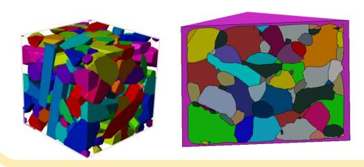
Technical Details: ■ 64 periodic grains + matrix (transverse-isotropic/isotrop) > 1'500 eqs. for PBC > 600 contact relations
